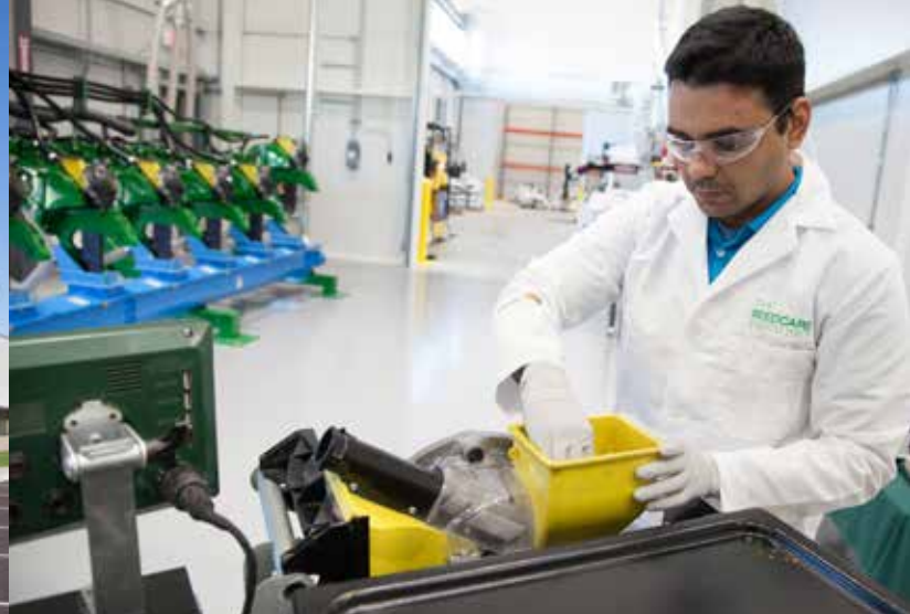
Top, left to right: Inside the facility in Stanton, Minnesota, Syngenta has incorporated casual meeting spaces for employees and visitors; Syngenta Seedcare experts evaluate the application performance of a seed treatment recipe using a lab batch treater; the new Seedcare Institute facility in Stanton, Minnesota, opened its doors in September 2016; Wanderson Oliveira, Seedcare platform specialist, evaluates planter performance of treated seeds. Bottom: Jars of seeds treated with Syngenta Seedcare brands represent a rainbow of colors.
